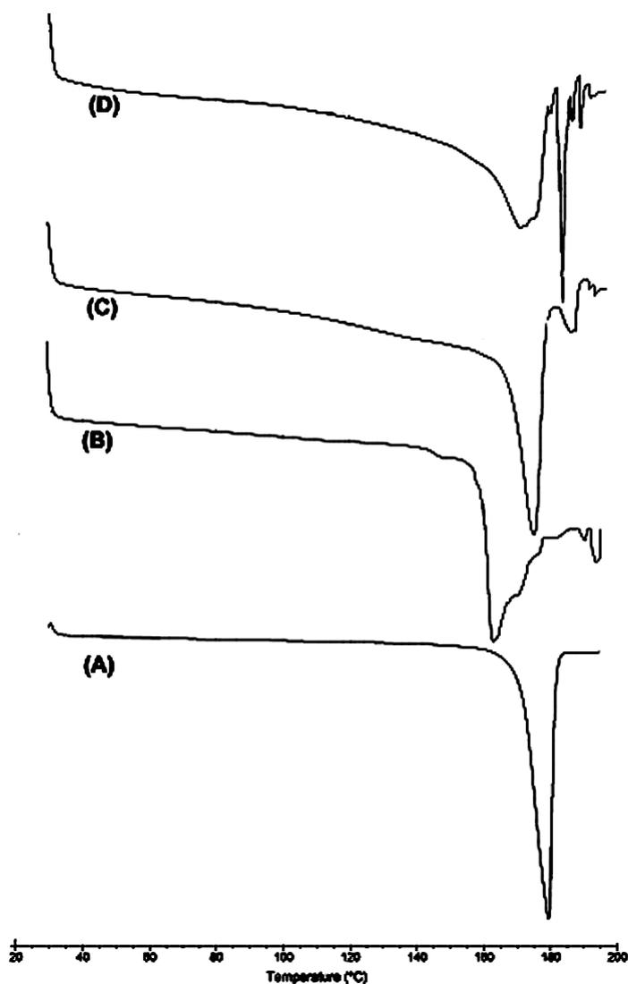
**Fig. 2.** DSC thermogram of pure curcumin (A), L- $\alpha$ -phosphatidylcholine (B), Physical mixture (C) and complex (D) of curcumin and L- $\alpha$ -phosphatidylcholine.
